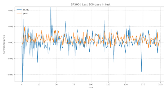
Fig. 7b Predictoin results for the last 200 days in test data. Model is trained with input_size=1 and lstm_size=128.
